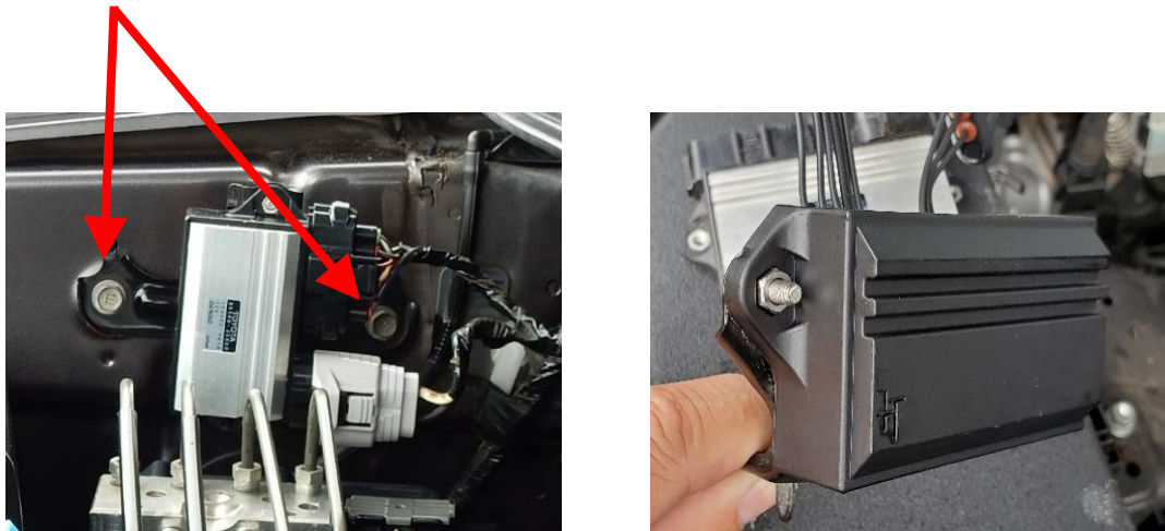
Figure 3 - Remove the factory AID from the Bracket and Mount the Gen-II unit.
