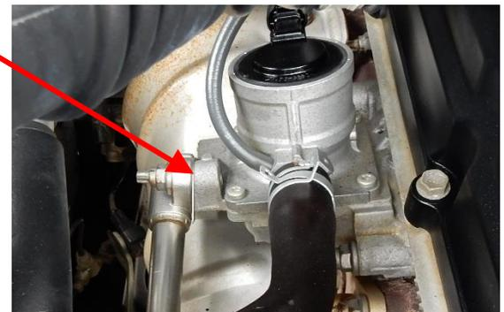
Figure 4 - Air Tube Removal
