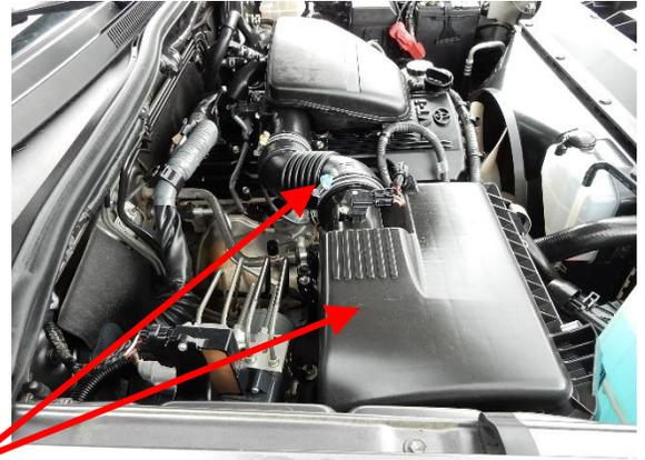
Figure 1 – Air Box Removal
