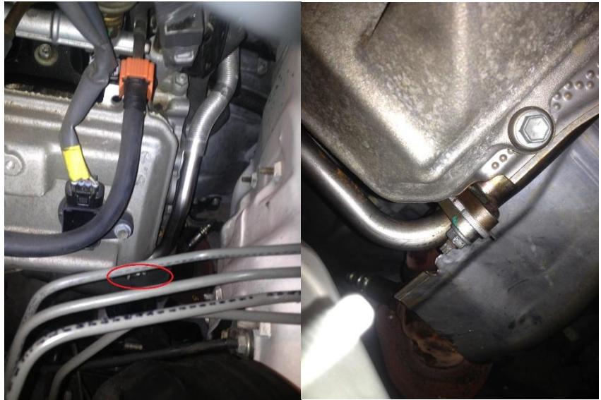
Figure 1 – For All 05-09 4.7L Vehicles (except 07-09 4.7L Tundra) Air Tube Flanges at lower firewall end of driver and passenger side cylinder heads.
