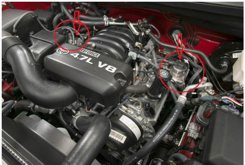
Figure 2 - 07-19 Tundra 4.7L block off plates install from topside between the airswitching valves and air tubes.
