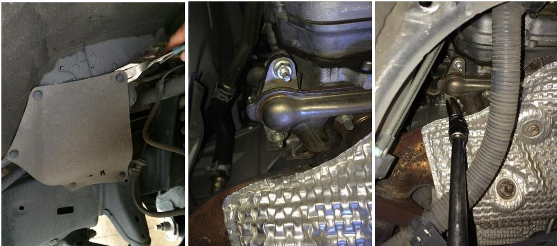
It is very important NOT to pry on the round portion of the tube or between the flanges which will cause damage to the mounting surfaces. Do not open more than needed to insert the plate. If either is damaged, you may create an exhaust leak.
