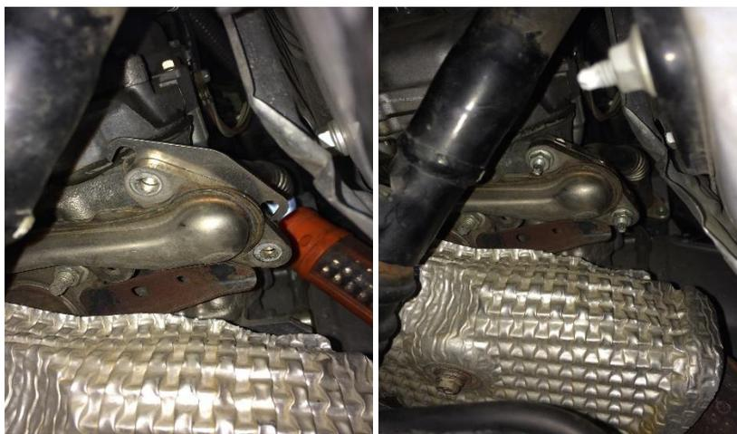
5) Once the plates are inserted and bottomed against the studs, tighten down both studs.
