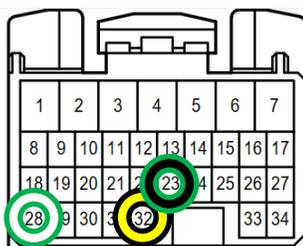
Figure 3 - Looking into the terminal side of connector E8 wire colors shown are coming out the back of the connector
