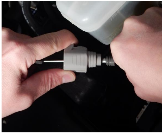
Figure 6 - Remove Terminal While Holding Terminal Tab Out Of The Way
