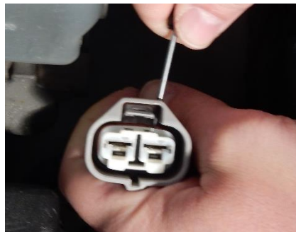
Figure 4 - Removing Terminal Lock
