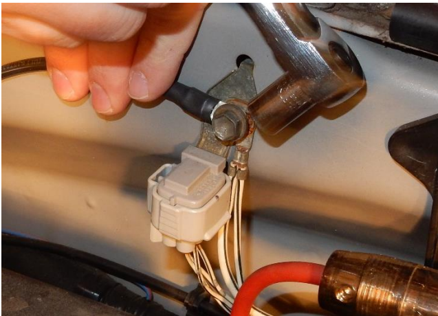
Figure 8 – Connecting the Pump Pack's GND Connection
