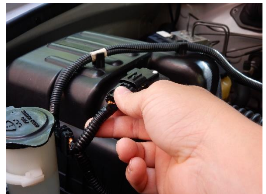
Figure 3 - Connect the Female Module Connector to the MAF/IAT Sensor
