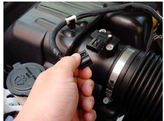
Figure 2 - Disconnect MAF/IAT from factory harness
