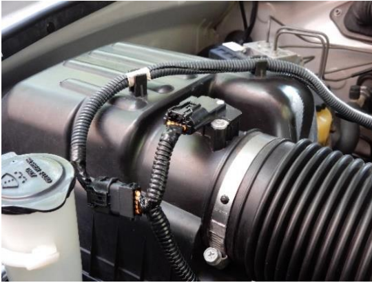
Figure 4 - Module Harness Installed
