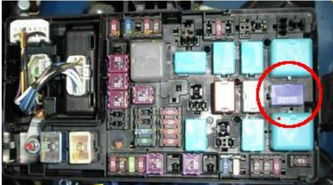
Figure 6 – Starter Relay Circled (labeled ST or STA on lid diagram)
