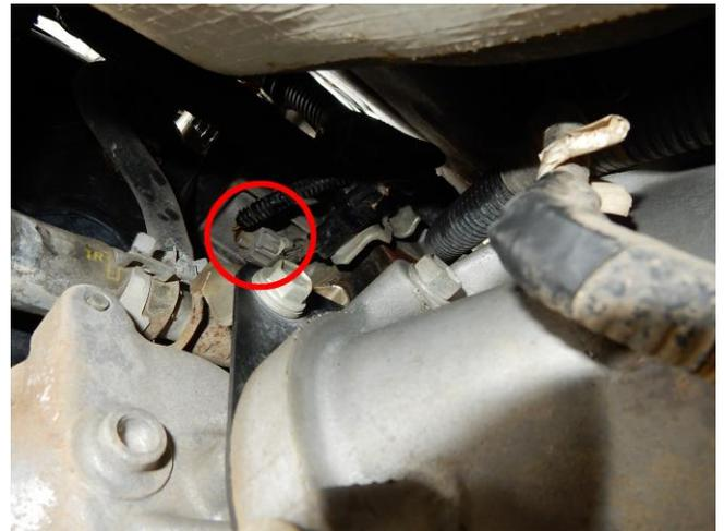
Figure 5 - ECT Connector at back of engine above starter
