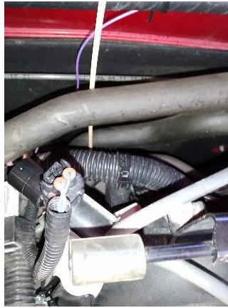
Figure 4 – Locate the ECT connector at the back of the engine. Shown by dowel.
