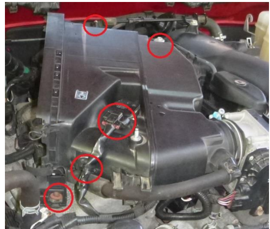
Figure 2 - Disconnect MAF/IAT from factory harness and remove the harness mount, mounting bolts and vacuum line.
