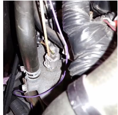
Figure 5 - View of ECT Sensor from Passenger Side Firewall
