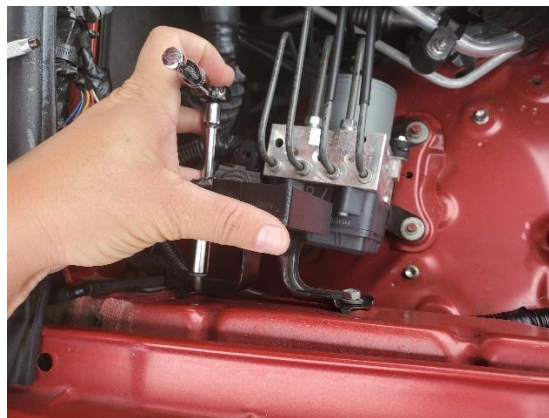
Figure 3 - Connect the wire harness to the Gen-II unit
