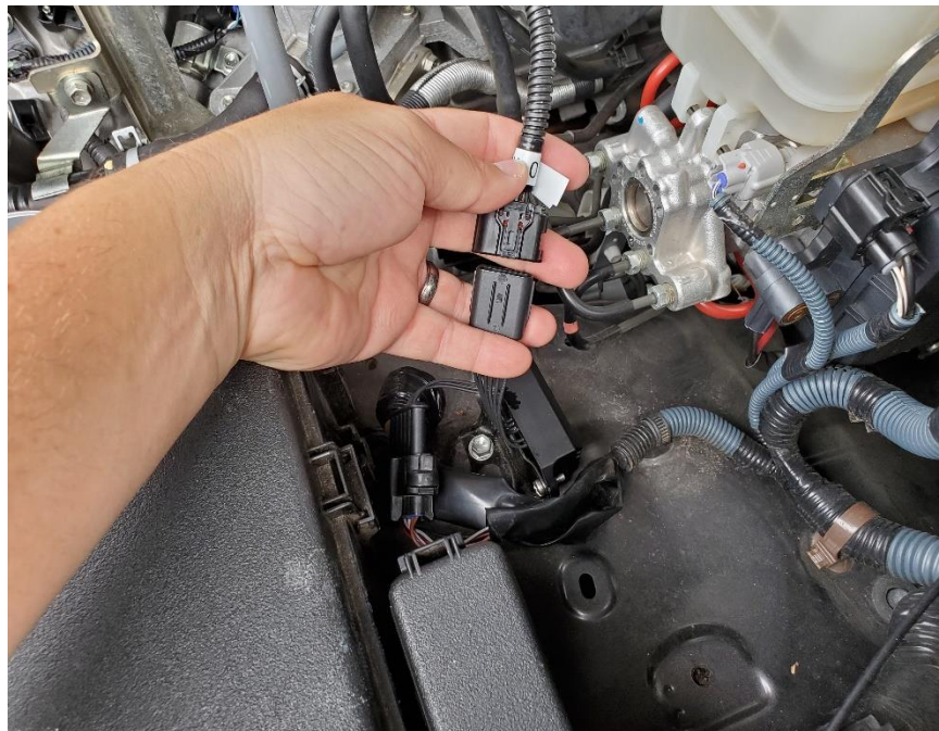
Figure 7 - Connect the wire harness to the Gen-II unit
