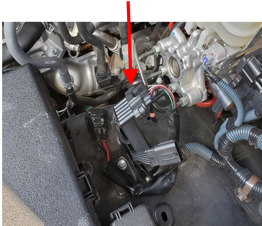
Figure 6 - Connect the six-wire connectors
