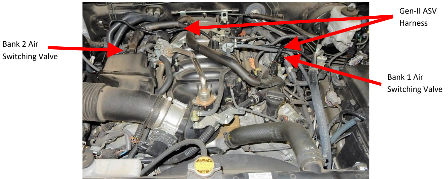
Figure 10 - Bank 1 ASV location and Gen-II harness routed over top of engine.
