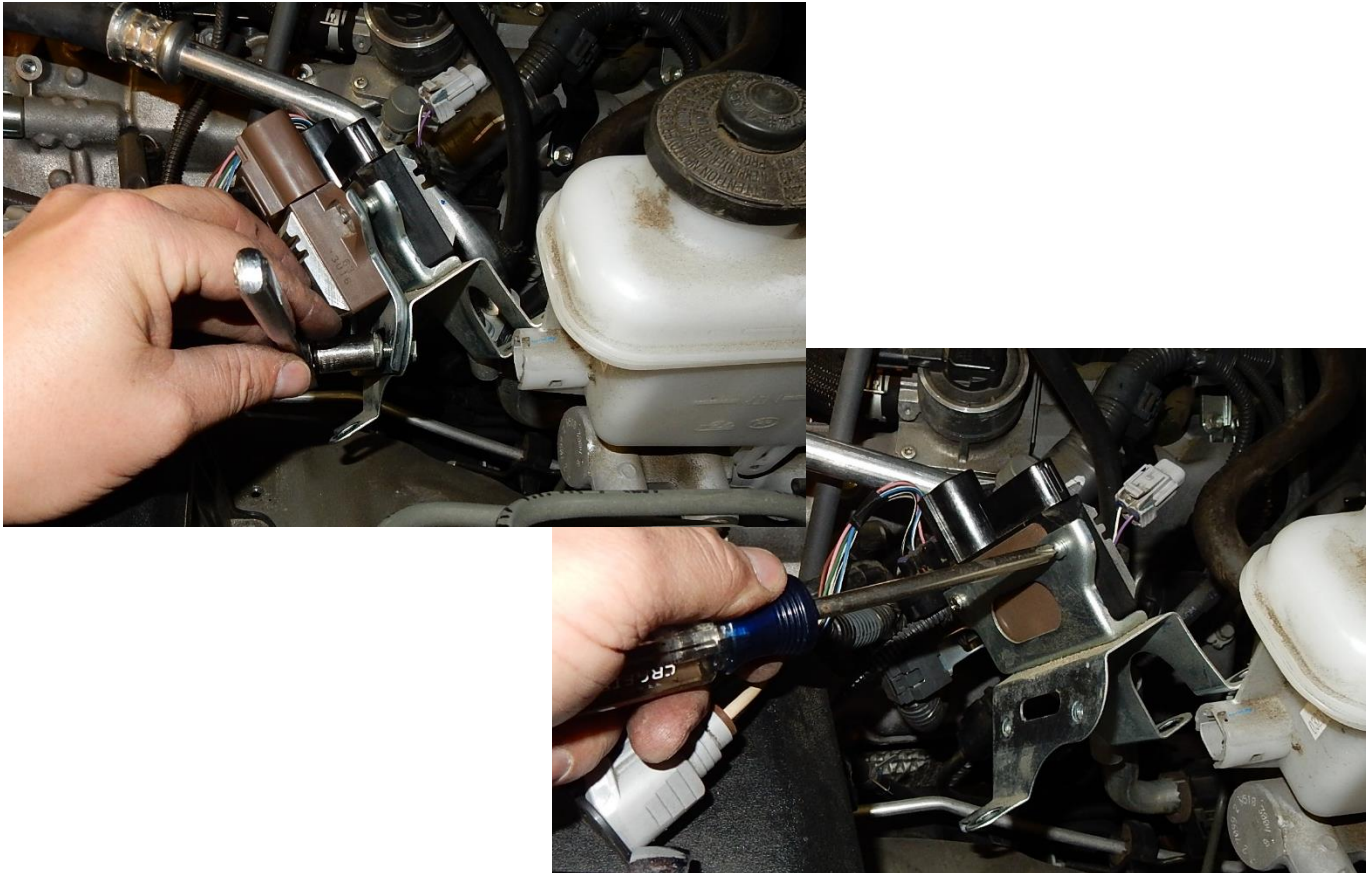
Figure 4 - Removing the air injection control drivers
