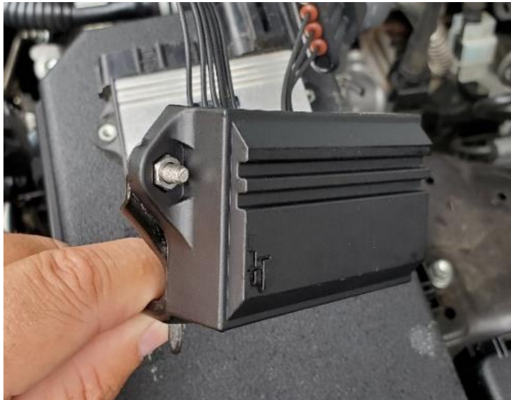
Figure 6 – Gen-II mounted to sub-bracket with included stainless screws/nuts
