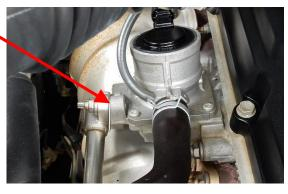
Figure 4 - Air Tube Removal
