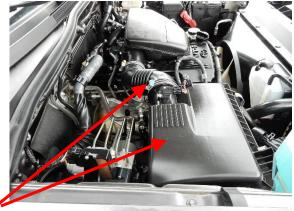
Figure 1 – Air Box Removal
