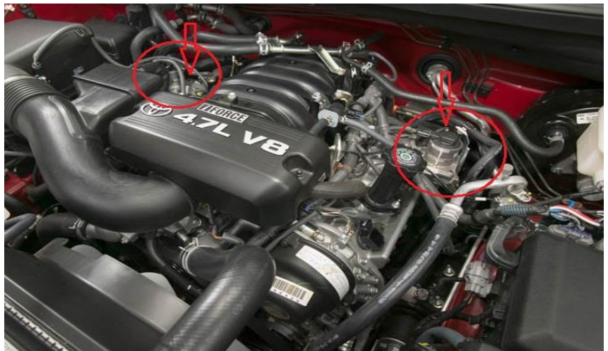
Figure 2 - 07-09 Tundra 4.7L block off plates install from topside between the airswitching valves and air tubes.
