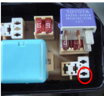
Figures 7, 8, 9 – Starter Relay, Twisted wire Connection to Correct Starter Relay Terminal, Starter Relay Reinstalled.
