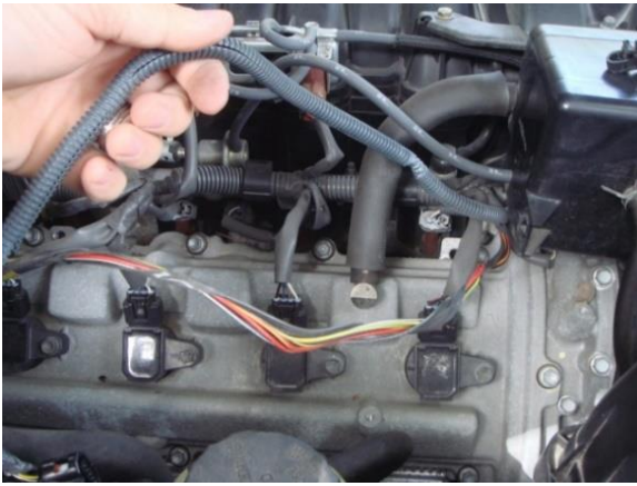
Figure 3 - Wire Pulled from Harness
