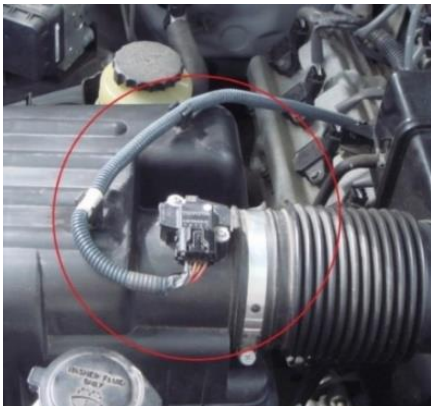
Figure 1 - IAT/MAF Sensor Location
