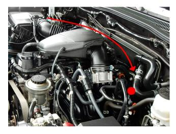
**Figure 2 - ECT Sensor Location**
