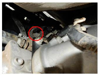
Figure 5 - ECT Connector at back of engine above starter
