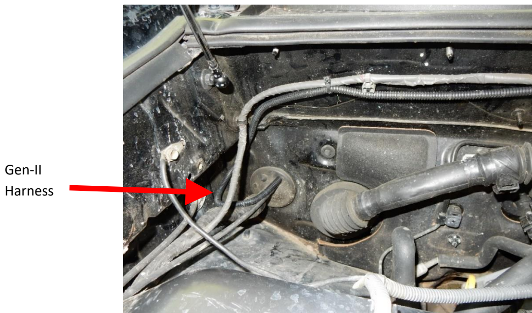
Figure 11 – Completed Under-Hood Gen-II Harness Installation.
