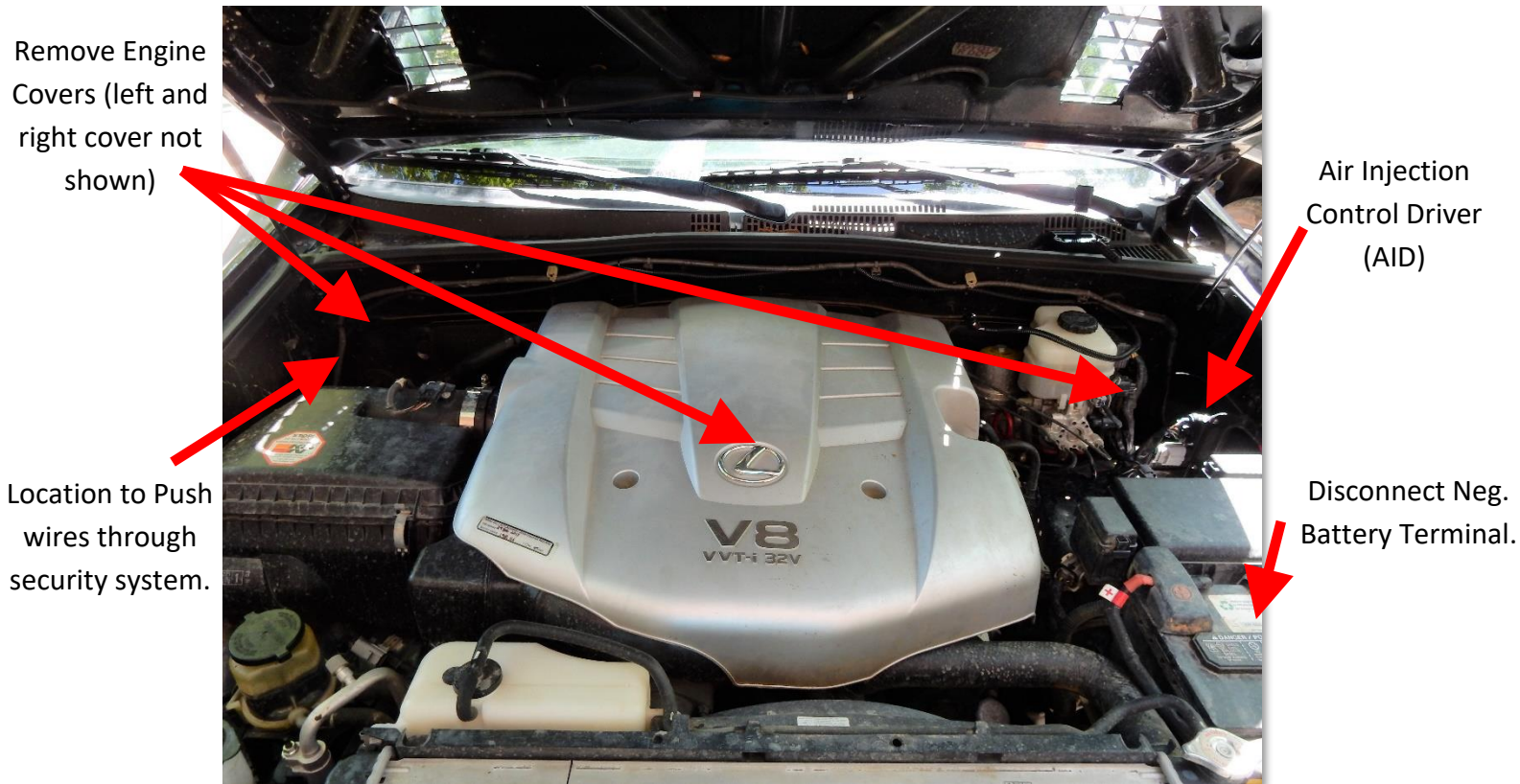
Figure 1 – 2005 GX470 shown. All vehicles covered in these instructions have the same layout as shown.
