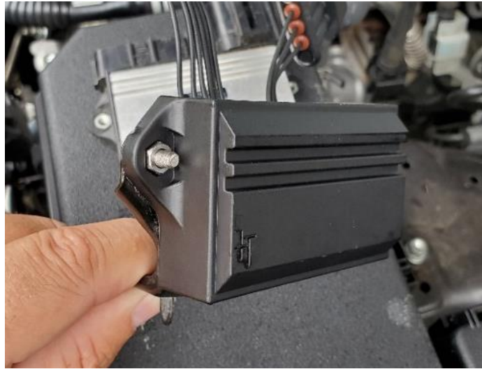
Figure 6 – Gen-II mounted to the sub-bracket for easier installation
