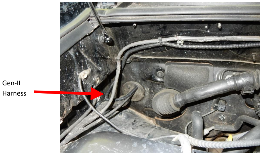
Figure 11 – Completed Under-Hood Gen-II Harness Installation.
