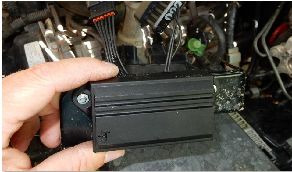
Figure 6 – Mount Gen-II Unit to sub-bracket.
