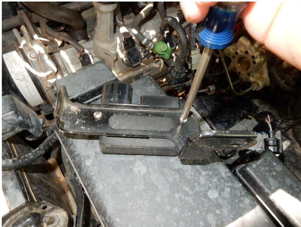
Figure 5 - Removing the AID from the Bracket.
