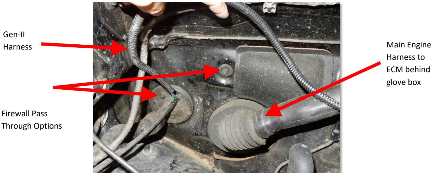
Figure 10 - Route End of Harness Through the Firewall for ECM Connections.
